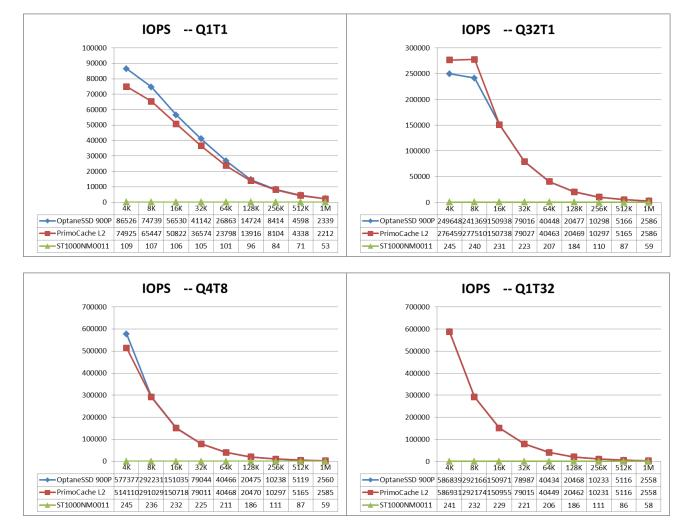
580,000. The test results show that **the highest IOPS value of 4KB random read is stable at nearly 590,000, which is even higher than the official rate of 550,000**.
